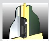
For ultimate security we offer a central ventlock. As you turn the key, part of the stile projects into a keeper located in the head. It allows sash to be locked in closed or partlyopen positions.
